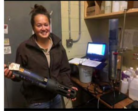
DNR technician calibrating continuous water quality meter for deployment in lake
